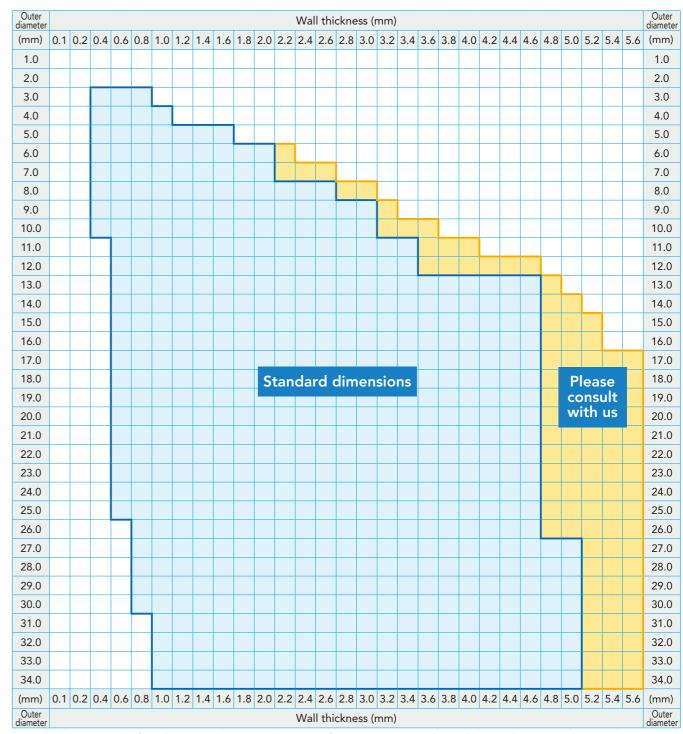
Remarks: The strength of steel pipes with an outer diameter of 34 mm or more and round bars with an outer diameter that exceed 100 mm requires separate consultation in accordance with ASME Sec. II-Part D SA-312 TPXM-19 and SA-479 XM-19 (1998).
