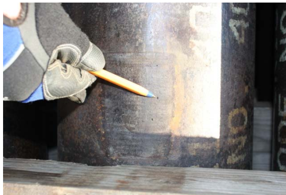
Pic # 4, Pitting initiation.
